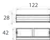
W-Type Joint Cover Material – PPCP B120
