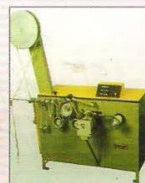
Spool winding machine
