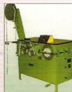
Roll winding machine
