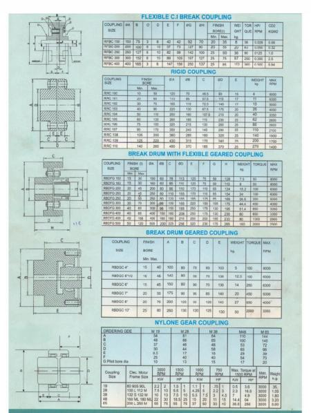
Brake Drum with Coupling details:
