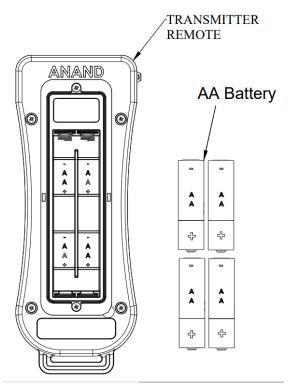
It's also worth noting that the Maks series remote control offers additional benefits such as installing 4 AA Batteries for Doubling the battery life, and improved productivity.
